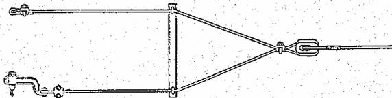
**Pull-Off Spreader with Pull-Over Yoke for Trolley Wheel**
