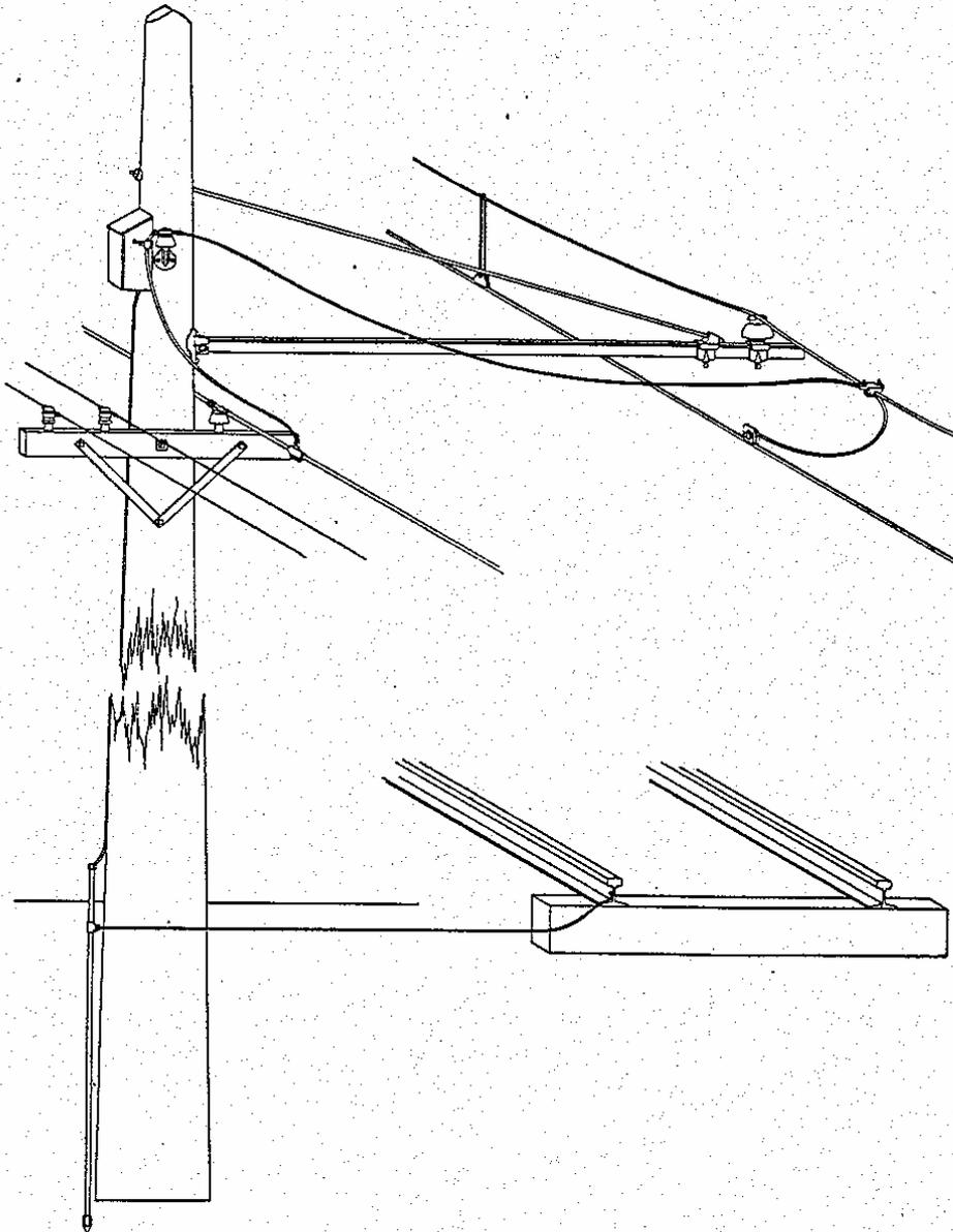
Showing Lightning Arrester and Feeder Tap
