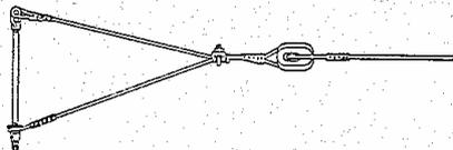
**Type CA Pull-Off Hanger for Wheel or Pantograph**
