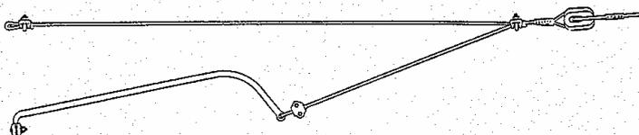
**Flexible Pull-Over for Pantograph**
