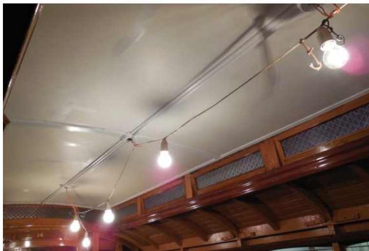
New painted ceiling panels fitted to A 14. The painted ceiling (as opposed to the varnished ceiling on A 15) is to represent a wartime repair.
