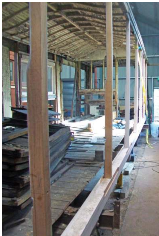
The new slats installed on the apron of the double-deck car. Peter Stock
