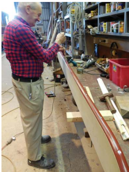
Bruce Lock fitting a D moulding to one of the new footboards for the Bib and Bub set.
