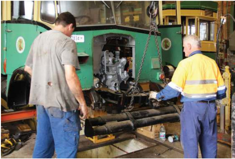
Bill and Craig reinstall the bumper bar on 22 February after the installation of the replacement engine. The bumper is made from three old tramcar axles.
