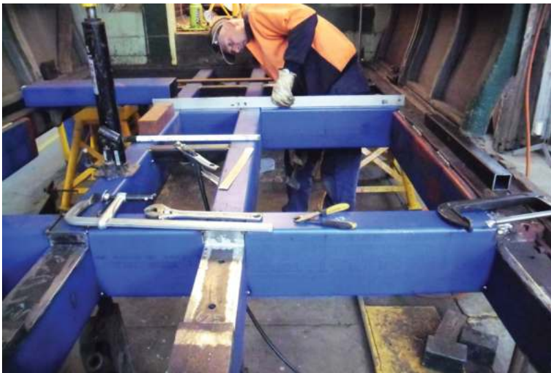
Mike Campbell working on the structural components of No. 7's cab floor.
