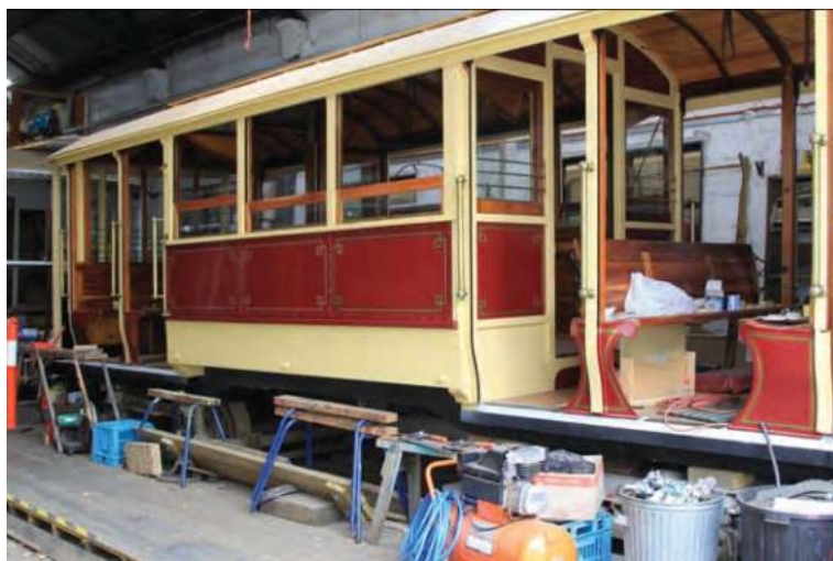
Launceston's first tram, car No. 1, is undergoing major reconstruction in the workshop.
