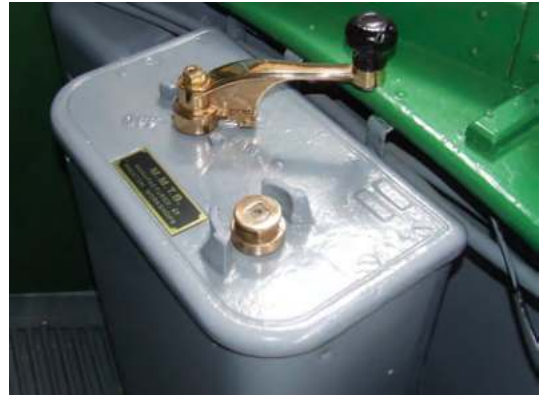
The refurbished RC2 controller in SW5 849 with the highly polished handle and the new MMTB RC2 plates fitted.
