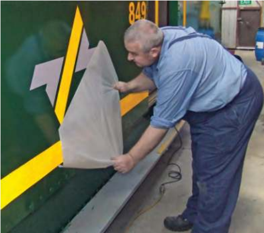
Kym Smith peels back the application paper to reveal The Met logo on the drop-centre side panel of SW5 849. The yellow on the logo, numbers and stripes is reflective under direct light but appears as a normal yellow when viewed in natural light.
