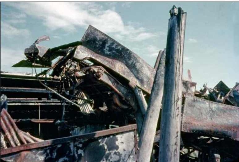
A dropcentre plate frame bogie hangs from its underframe on 14 April 1963. H.R. Clark
