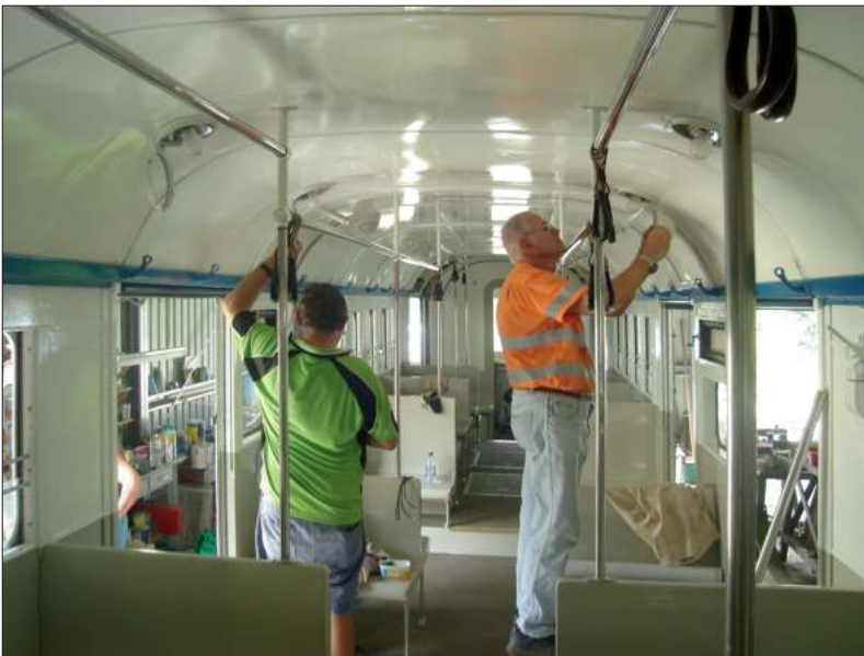
Pat Bourke and Ian Brandt complete fitting reflectors and lamp shades inside car 400.
