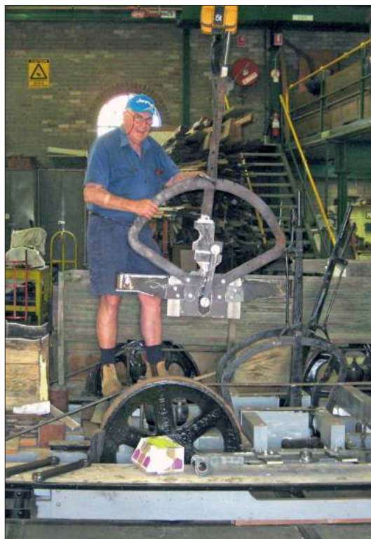
Warren Howlett prepares to install the dummy grip in car 322 with the aid of the overhead crane on 7 November. Mick Duncan
