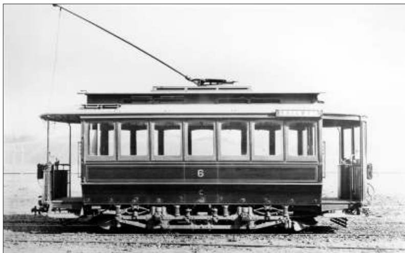
An enclosed seven-window saloon (C class car) at Moore Park. The enclosed saloon cars built for the George Street electrification were fitted with destination boxes with linen rolls. Cars for the Edgecliff-Rose Bay electrification had no destination indicators, or were fitted with roof-mounted four-sided blocks showing destinations.
