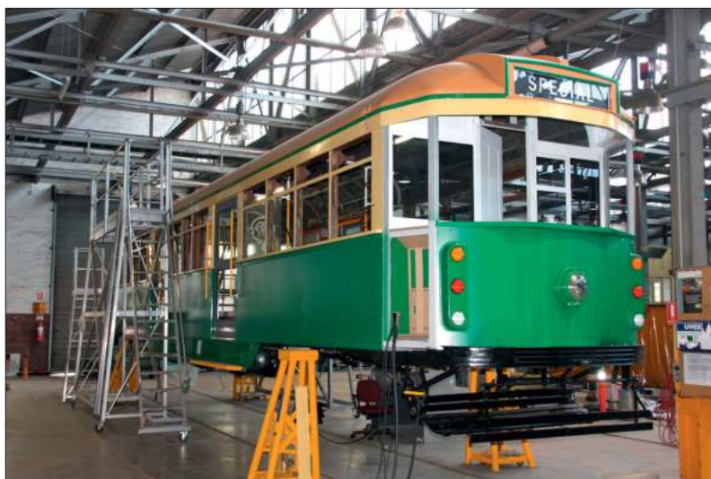
Car 946 undergoing its overhaul and upgrade at Preston Workshops late in July. It appears that the door on one side of the driver's cab – the right hand side facing the direction of travel – will be blocked off and replaced by an electrical cabinet below window level. The tram has yet to be painted in City Circle colours.
