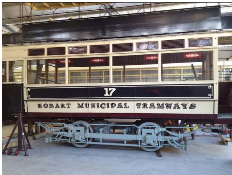
Hobart tram 17 with its new truck on 18 June.
