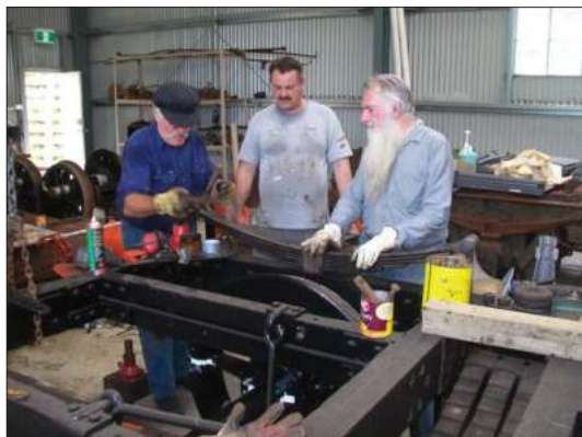
Undertaking the final assembly of a bogie from end platform carriage LFA 179 in February 2012. The other bogie will now be thoroughly overhauled. Pictured left to right are David Lewis, Craig Connelly and John Webb.
