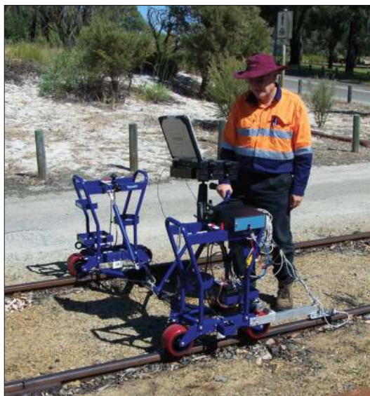
The hand-propelled unit designed to measure track geometry, under trial near the Village road crossing on 29 March. Note the laptop computer on top.
