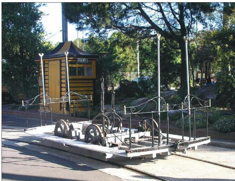
Another view of Melbourne cable grip car 322 on 3 December. It has since been fitted with lifeguards. Work continues on completing the end aprons. Richard Jones
