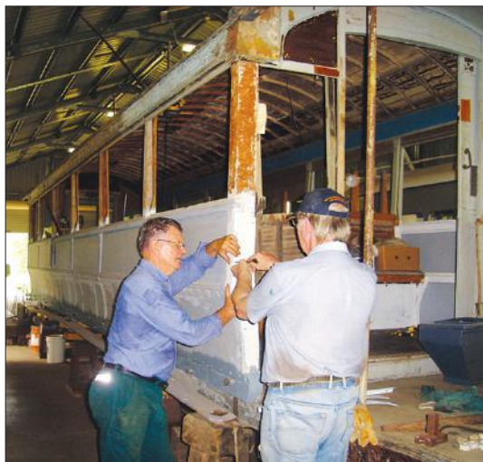
Bevan Burnes and Darryl Soden complete the re-installation of side panels on Dreadnought 136.
