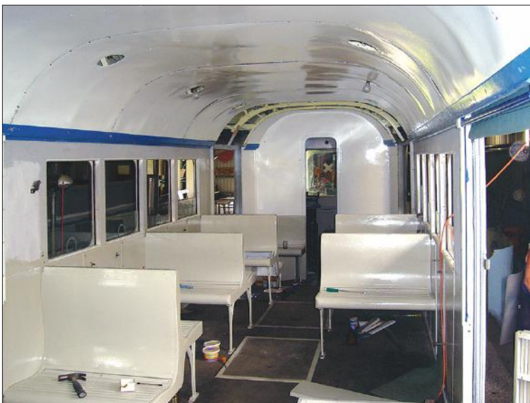
Re-installed seats and ceiling panels in the car. Peter Hyde
