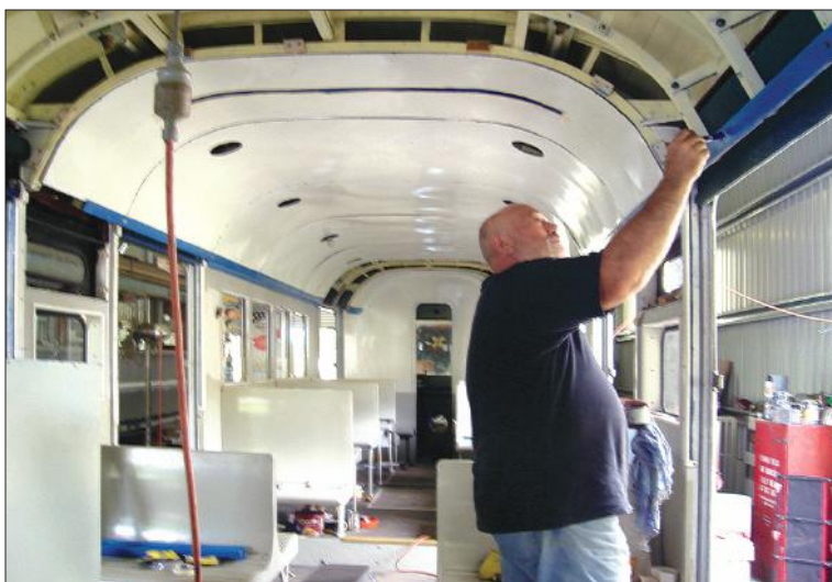
Bevan Burnes and Darryl Soden complete the re-installation of side panels on Dreadnought 136.
