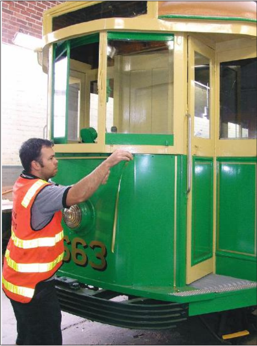
Heath from Signarama Bendigo applying the numbers and lining to the front of W3 663.
