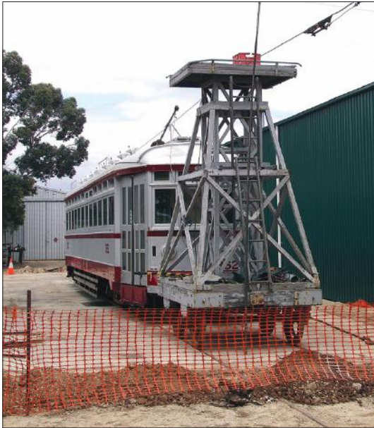
H 362 and the tower wagon act as a pit cover and overhead support while work progresses on the new shed.
