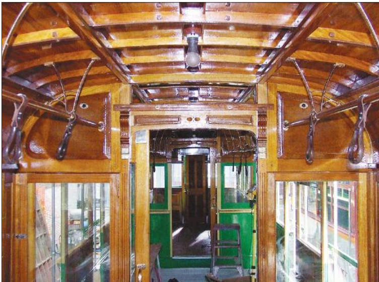
The varnished interior of W3 663 looks resplendent with the installation of seats and remaining fittings. Anthony Smith
