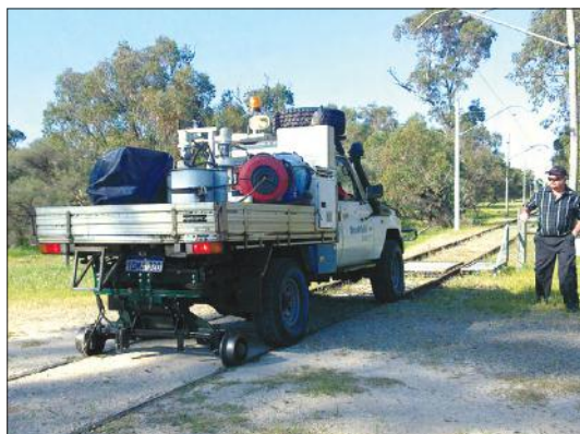
A hi-rail equipped Land Cruiser is tested on the tramway at the Horse Swamp cattle grid by Trac-west Machinery on 6 October. Simon Mead
