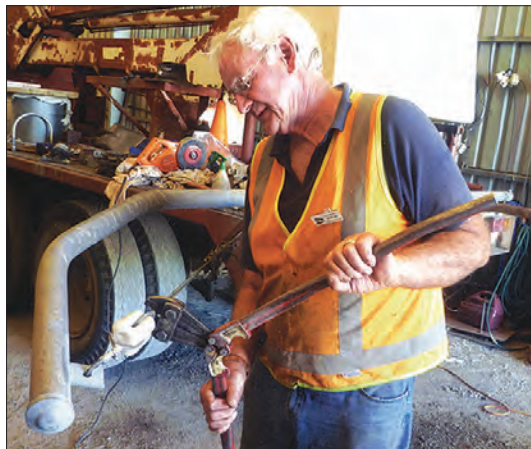
Duncan McVicar fitting out overhead bracket arms on 8 December 2010, ready for installation on the new steel traction poles.
