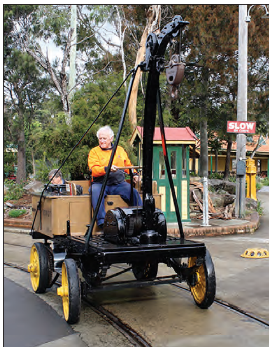
The Sydney Tramway Museum's Sprague GE battery workshop crane was tested on 1 June using a lead from the workshop motor generator set. The little crane operated flawlessly.
