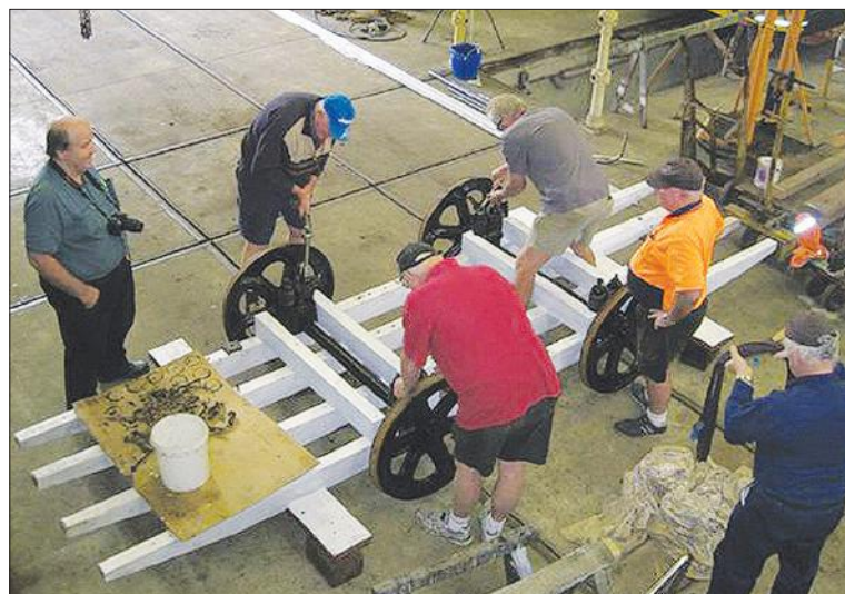
The new frame for Melbourne cable dummy 322 had its wheels fitted on 20 April.
