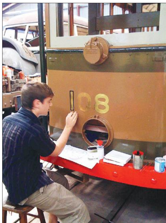
Joseph Spinella applied gold leaf numbers to the southern end of OP 1089 on 9 April and is proceeding to outline them in black. Side numbers were applied on 16 and 23 April. Numbering the north end of the car had to wait until the car could be moved to obtain access room.
