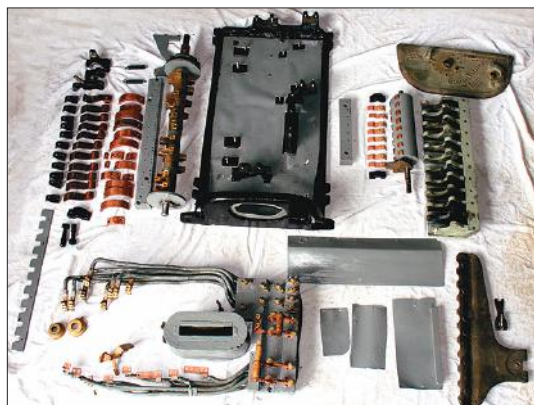
An exploded view of a K10 controller for dreadnought 136. Ken Howard
