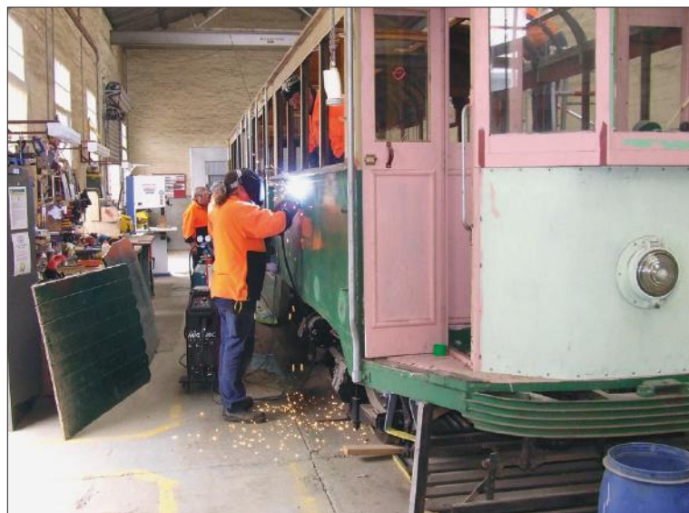
Scott Kendall mig-welds closed the former advertising panel screw holes on the side panels of W3 663, assisted by Sam O'Brien.
