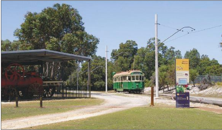
W2 393 passing the two newly-erected steel traction poles near the Tractor Museum. The rotted timber poles they replaced are lying beside the track. Michael Stukely
