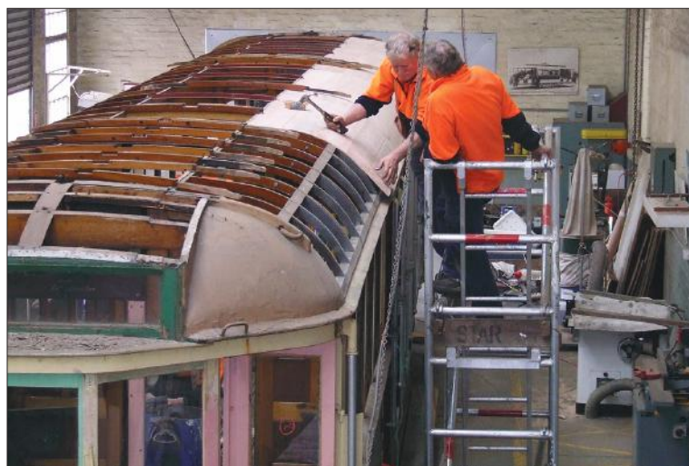
George Stirling and another member of the coachbuilding team install the plywood roof sheets on W3 663.
