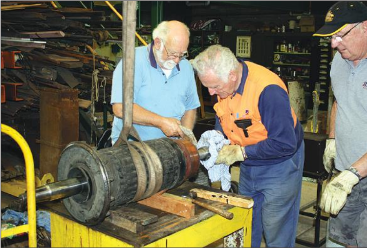
Alan Lark and Terry Thomas prepare to assist Bill Parkinson with installing a sleeve onto the armature of a motor to be used for C 37. Martin Pinches
