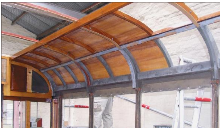
The first replacement plywood roof sheet installed on W3 663.
