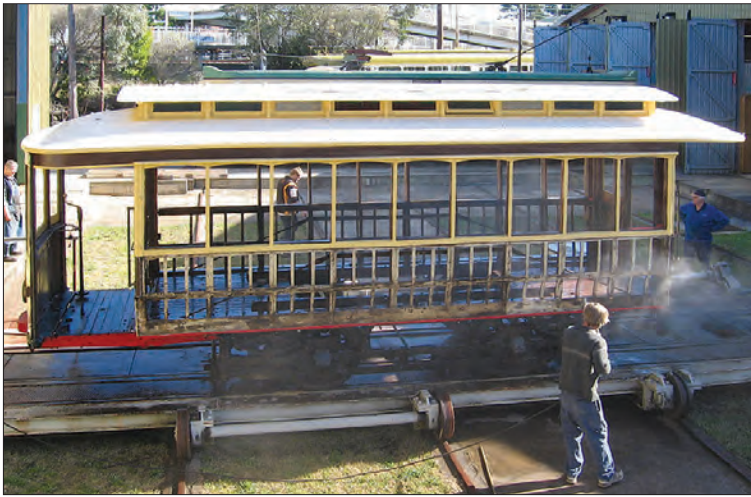
The floor area of C 37 was water blast cleaned on 16 June in preparation for work to commence on timber repairs.
