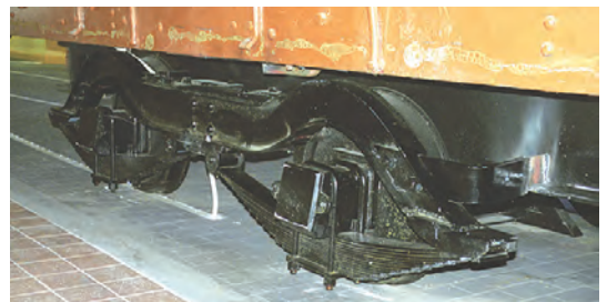
The dummy bogie constructed for the car by the Sydney Tramway Museum's Wednesday workforce. Dale Budd
