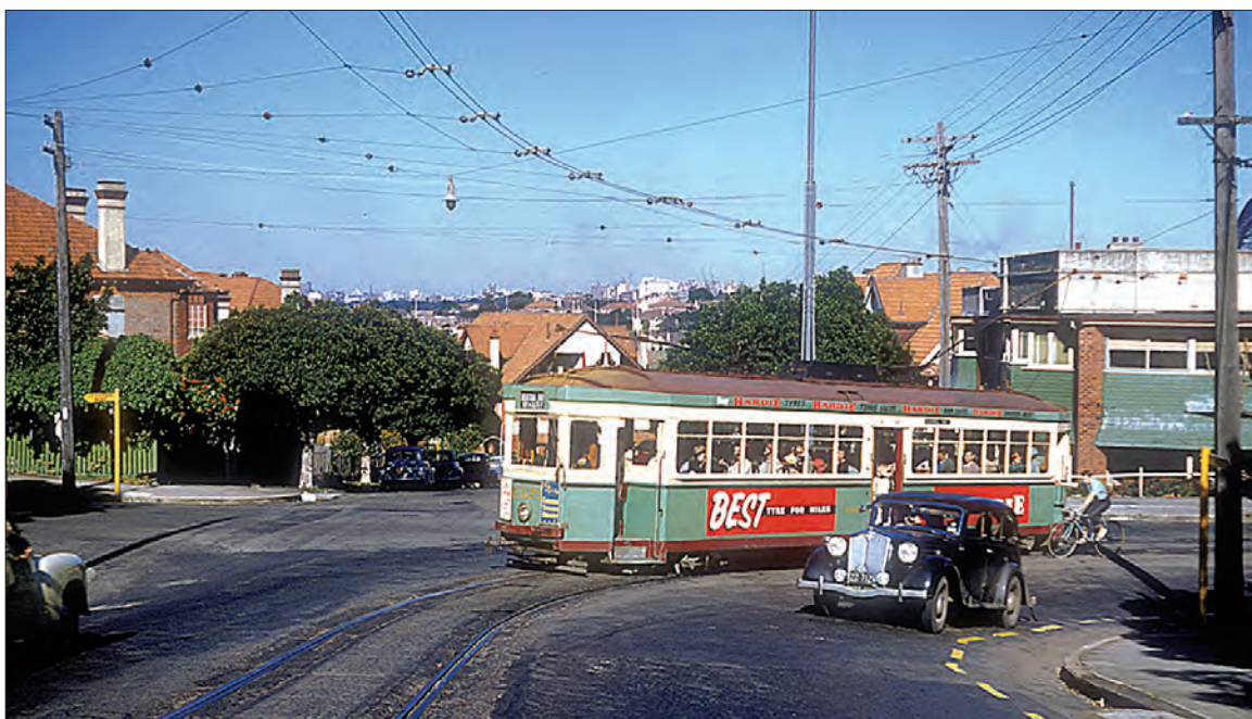
Sydney R1 class 2029 turns from Kurraba Road into Wycombe Road, Neutral Bay on its journey from the ferry wharf to Neutral Bay Junction in the 1950s. 2029 is fitted with roof-mounted dynamic braking equipment to assist its journey down the steep grade from the junction to the wharf.
