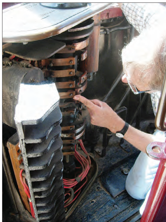
Mike Bosworth examining the controller contacts in car No. 111 following adjustments by Andrew Gilbertson.
