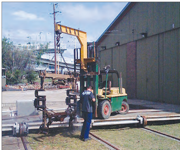
Craig Parkinson steam cleans one of the Brill 22E bogie frames from Ballarat 37.
