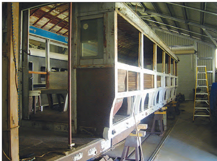
Dreadnought 136 showing repairs to the timber structure in preparation for installing the new curved side panels.
