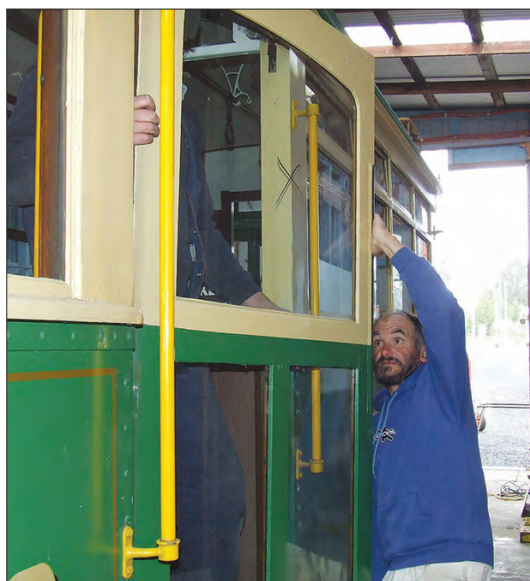
Arthur Ireland assists Anthony Smith (inside the tram) to remove one of the sliding doors from SW5 849. Jacqui Smith
