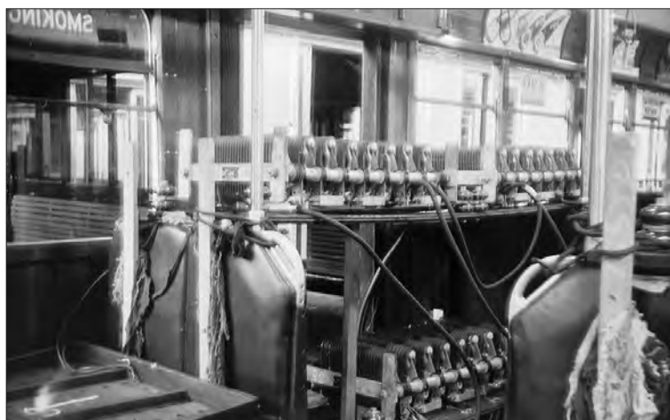
The dynamic brake equipment being installed in R1 1999, seen from an adjacent O class car.
