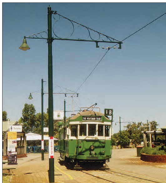
SW2 No. 426 at the Village tram stop on 7 January, showing the newly painted dark green steel traction poles with added (small) finials and street light brackets, as well as the newly painted Perth-style Tram Stop signs on the poles.
