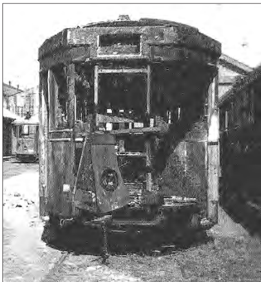
The end of the tram damaged in the collision with the truck and subsequently burnt out. Leon Manny
