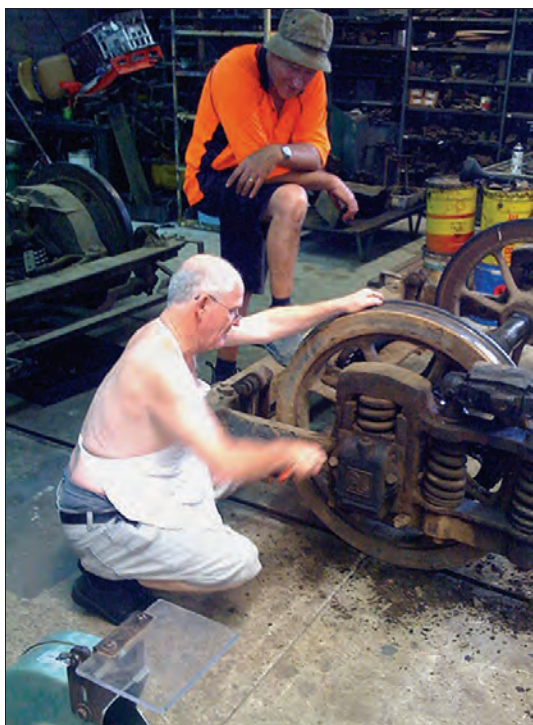
Dennis O'Brien is watched by Mike Giddey as he cleans accumulated grease and grime from the 22E truck from Ballarat car 37.
