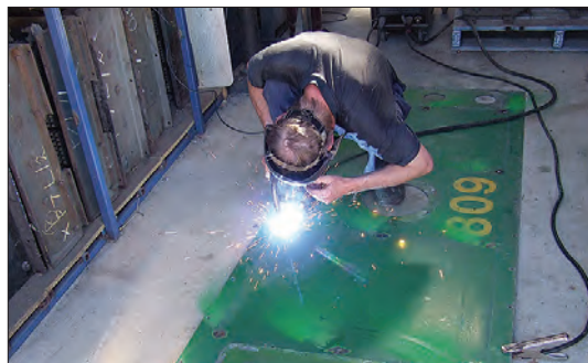
Frank Schroeders welds closed the advertising panel screw holes on the apron from SW5 809 prior to it being prepared for use on SW5 849.
