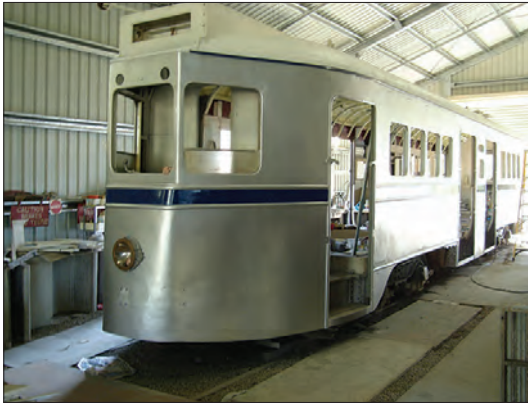
Restoration of prototype FM No. 400 is progressing with external painting almost complete.
