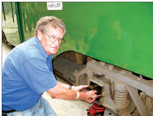
Frank Cuddy withdraws the axle bearing on Nagasaki 1054 for inspection.
