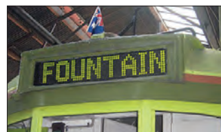
The dot matrix destination display fitted to car 34.
