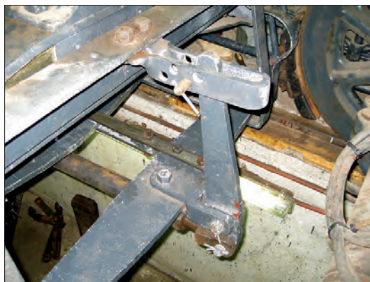
The Brill 27G bogie showing the new turnbuckle, brake beam and blocks, and beam guide to keep them parallel.
