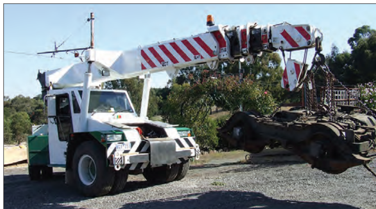
The Franna crane makes light work of moving a No. 15 truck from the main line to the storage container. Jacqui Smith
