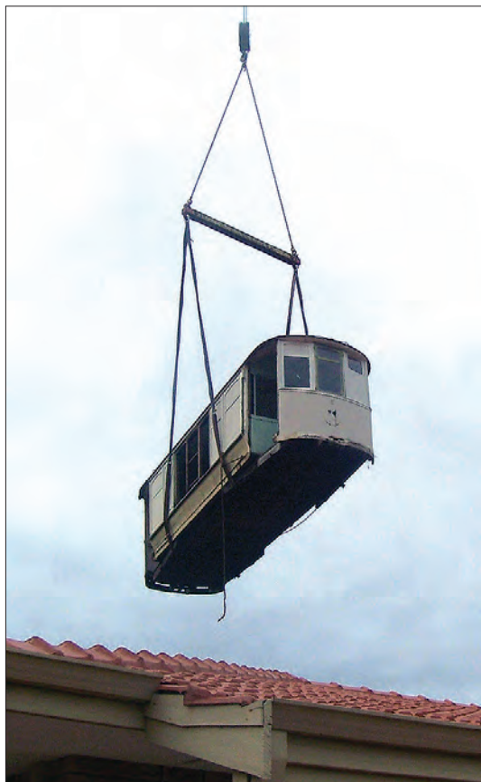
The 'flying tram' in Leslie Street, Mandurah on 26 July. B 43 is lifted high over the house from the far end of the block to the street in one manoeuvre by the 200 tonne crane, for loading onto the semi-trailer for the move to Perth. Graham Lees
