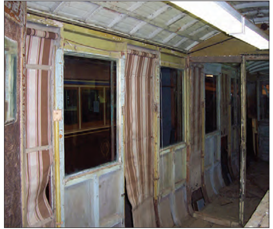
Interior of ESKo 22: after the big clean out we found that the pull down blinds, except for the lower 400mm or so, were still intact and working.
