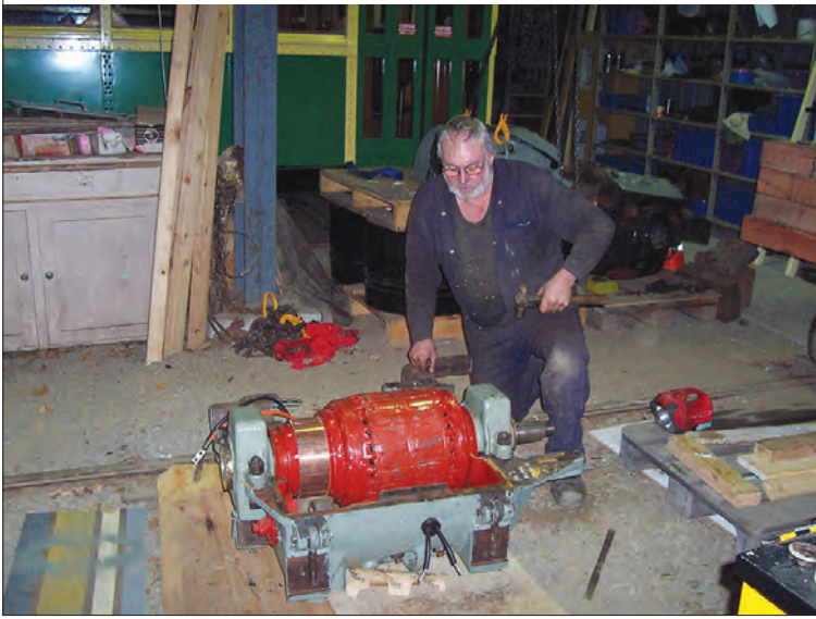
Alan Snowball working on the assembly of one of No. 14's armatures on 11 June.
