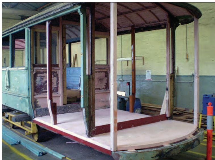
Launceston 14 with its new summers and flooring. Bendigo Tramways
