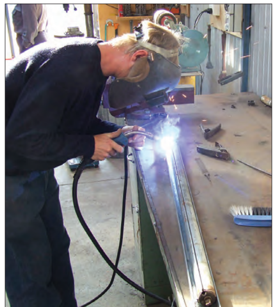
Frank Schroeders mig-welds one of the weather blind rollers for L 103. Rollers from W2 class trams were extended to the length required for the L class.
