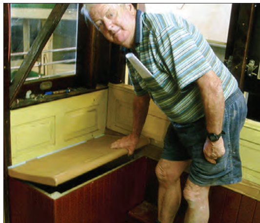
John Davies tests one of the four new end box seats he made and fitted into WAGT E class 66.
