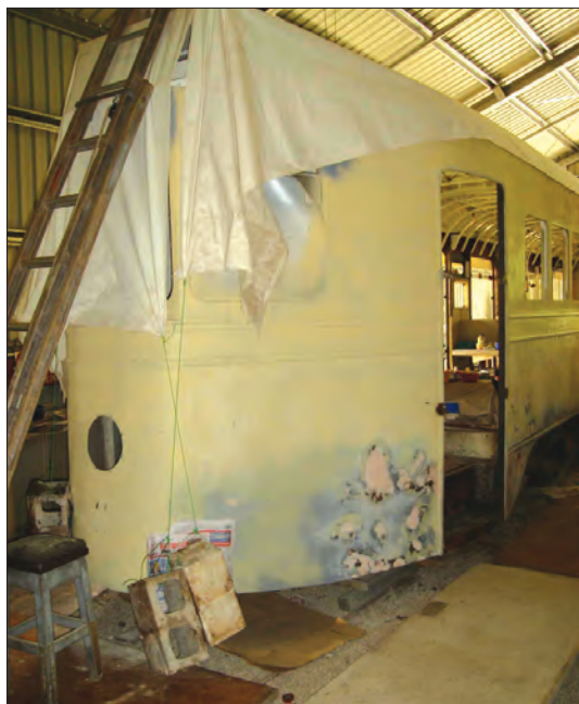
Stretching the new roof canvas on car 400 was aided by hanging concrete Besser Blocks on 3 February 2009.
