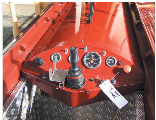
The control panel and engine cover of the new grip car. Portland Cable Trams
