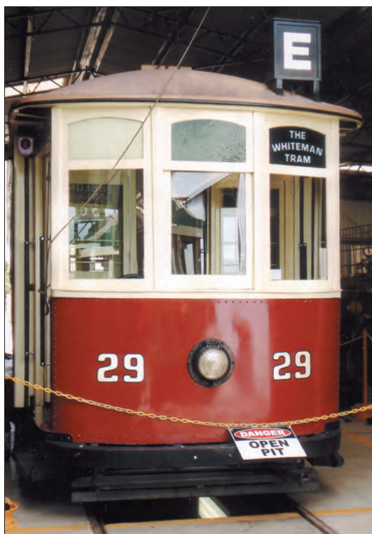
Fremantle 29 over the pit (western end) on 26 November ready for a periodic service, after running in under power using the wandering lead.
