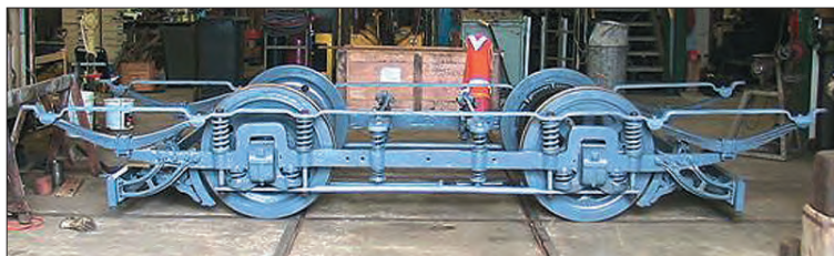
The truck for D117 was assembled on 28 August and the wear in the axle box hornways was measured for new wear plates to be made. The truck frame has since been lifted again to allow this work to continue.
