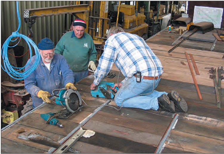
Three of our Wednesday team, Alan Leask, Warren Howlett and Rainer Nickel install more deck boards on ballast motor 42s on 17 September.
