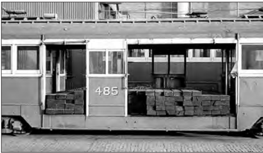
The centre section of No. 485 showing the rudimentary changes made for its sleeper-carrying role.
