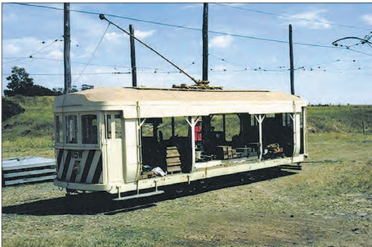
Sleeper transport tram No 15W on the main line at Bylands, ready to be restocked with sleepers for trackwork further down the line.
