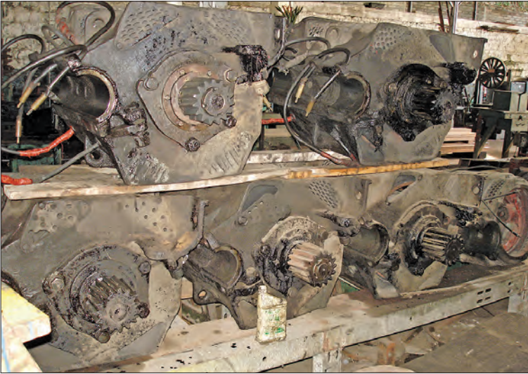
Overhauled electric motors await fitting into the trucks of out of service cars. Ian Dunn
