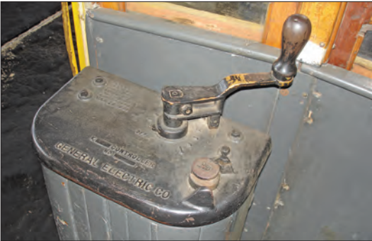
A General Electric controller dating from 1908 provides control for the Carioca cars. Ian Dunn
