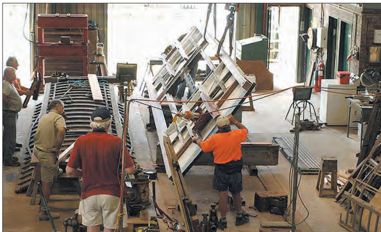
The underframe of D 117 was turned over on 15 December to facilitate fitting underfloor equipment. Matthew Geier
