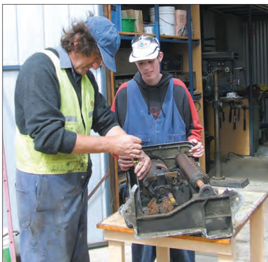
Anthony Smith and Daniel Edwards dismantle a damaged RC2 controller to provide parts for use in SW5 843.
