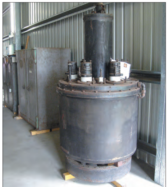
The Brown-Boveri rectifier and the safe in position. Peter Hyde
