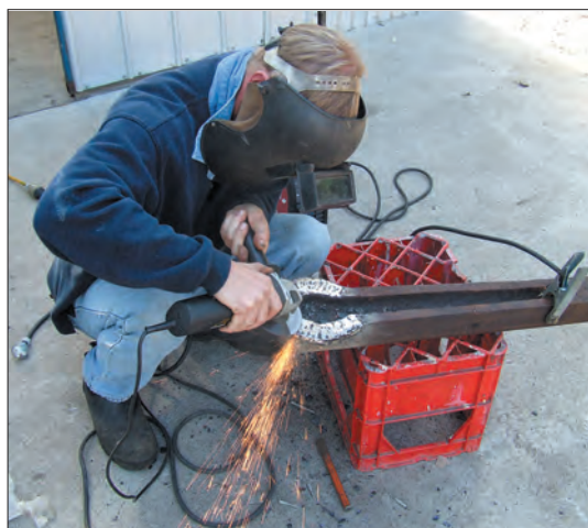
Frank Schroeders cleans up the welding on the heel of the Road 5 point blade. Anthony Smith
