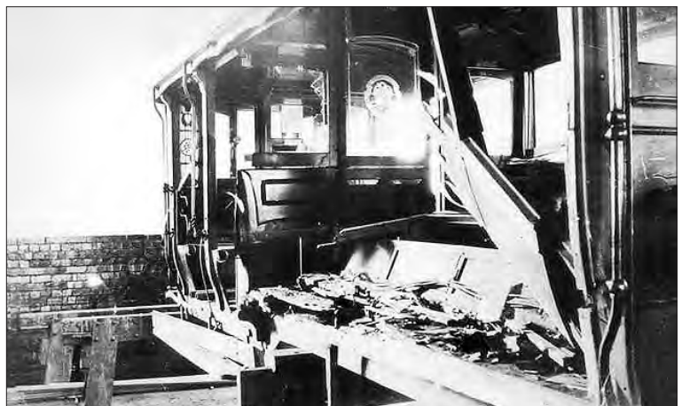
MMTB No. 65 after the 1923 Deepdene derailment, and prior to repairs.
