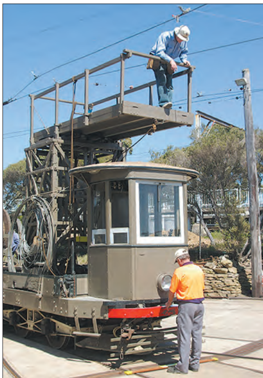
Tom Tramby assists David Rawlings with overhead wiring adjustments in the depot yard. David has constructed a laser unit to help pinpoint the relationship between track and overhead.
