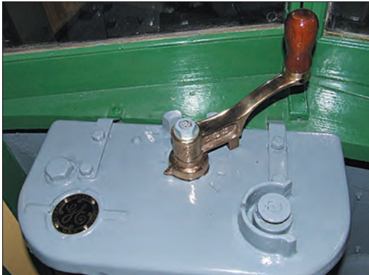
The newly installed GE badge on the K35 controller in L 103. Anthony Smith
