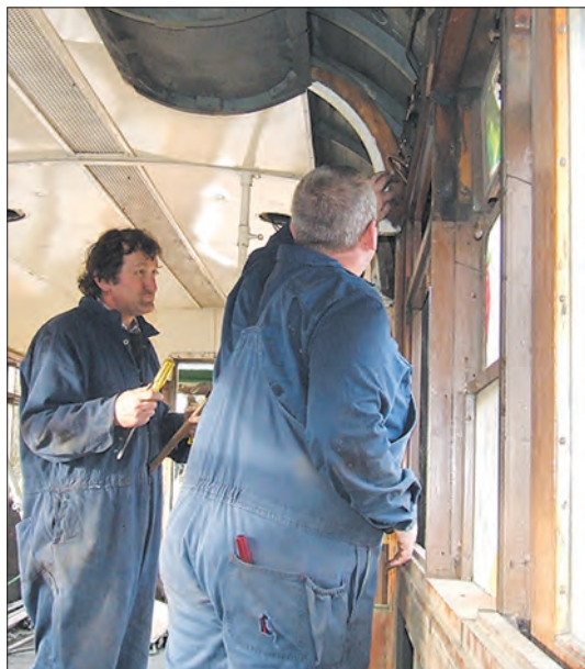
Kym Smith and Anthony Smith remove door engine components from W7 1008. Jacqui Smith
