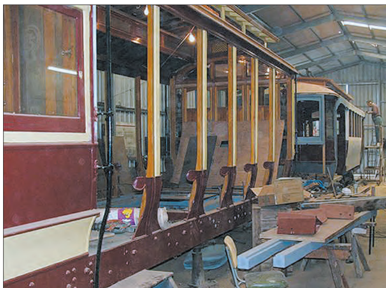
Cars 118 (front) and 14 being worked on in the body shop. Timber and cleaned up steel work for car 14 is next to car 118. Chris Summers
