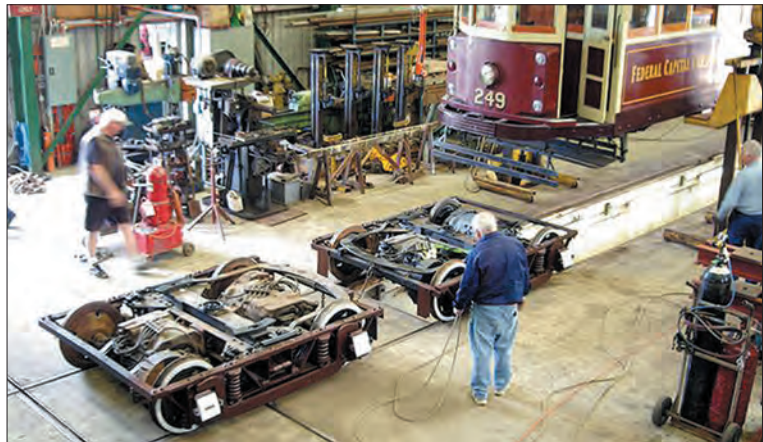
The replacement bogies are driven under the car on 30 May. Martin Pinches
