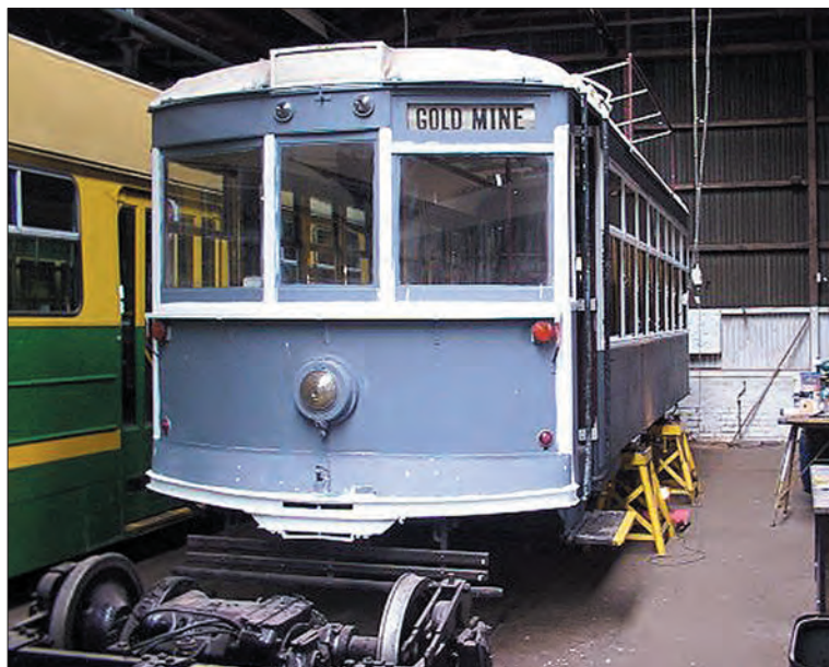
Birney 30 is standing on trestles in the paint shop whilst its truck is overhauled. Its body is in undercoat. Bendigo Tramways
