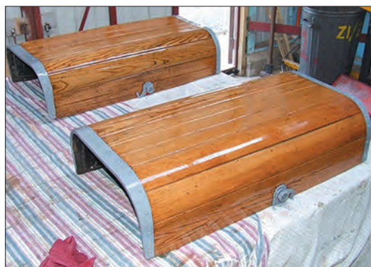
Controller covers being varnished for L 103. Anthony Smith
