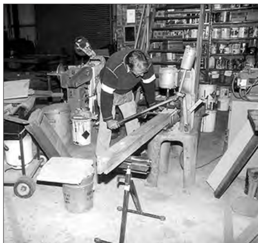
Geoff Spaulding mortises the new underframe bearers for D 117. Howard Clark
