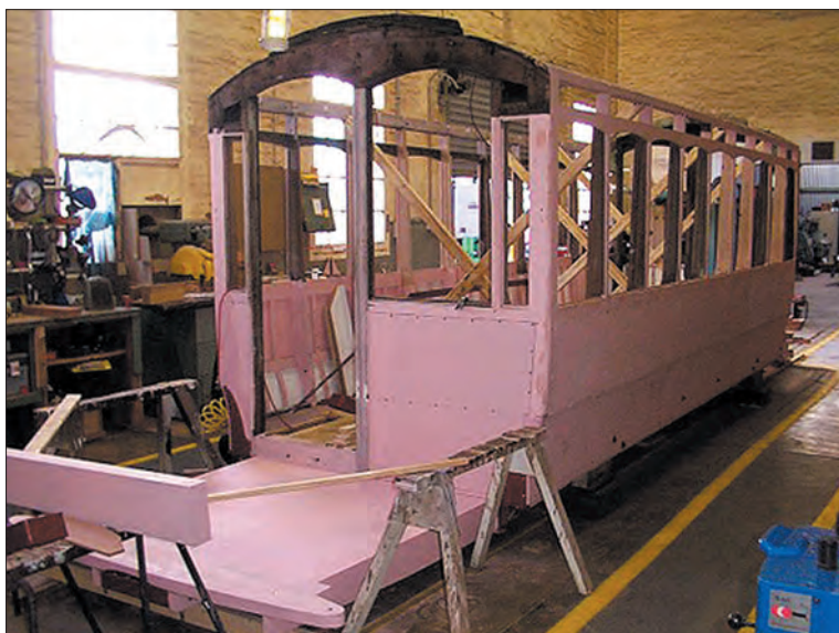
Sydney C 33 now has its end platforms and side panels (above and right).
