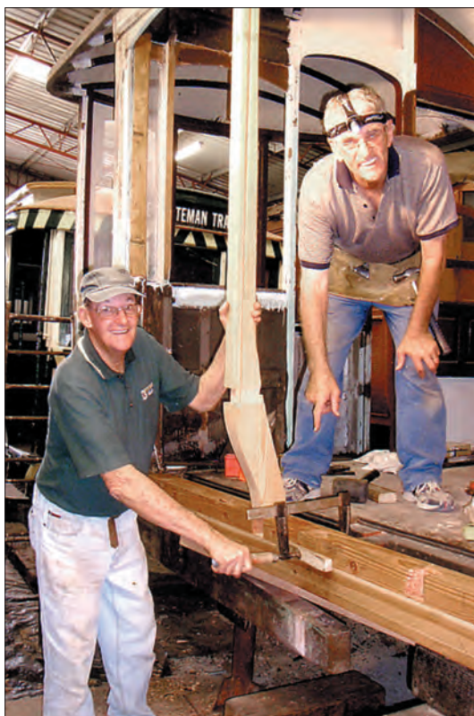
It fits! Jack Kendall (left) and Bryan Adcock installing a new side pillar in Perth B class No. 15, on 20 June. Ballarat 31 can be seen behind.
