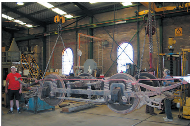
The Brill 21E truck from D 117 was moved on 6 June by workshop crane to enable it to be dismantled and cleaned.
