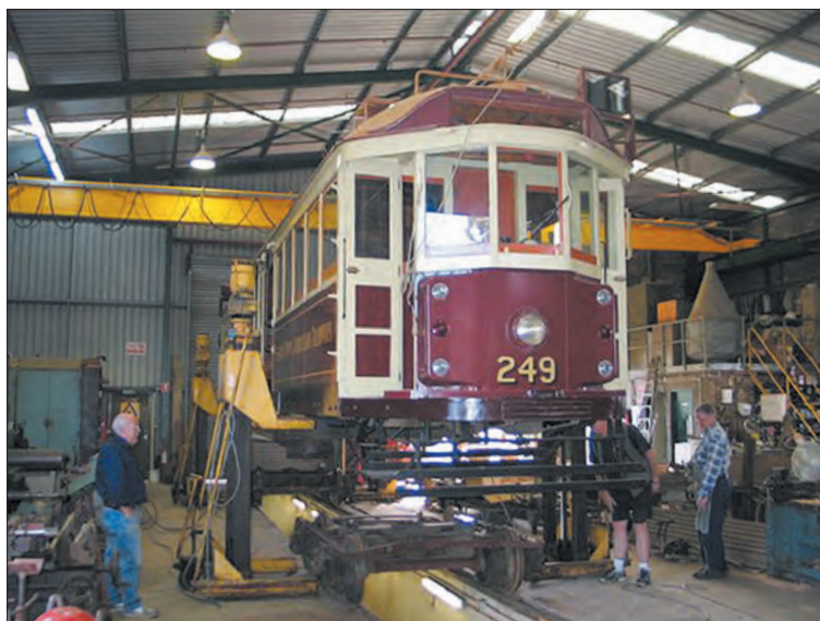
The replacement bogies are driven under the car on 30 May. Martin Pinches
