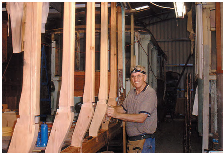
Bryan Adcock with the new side pillars and longitudinal beam installed in Perth B class No. 15, on 20 June. The body of Fremantle No. 14 is visible behind.
