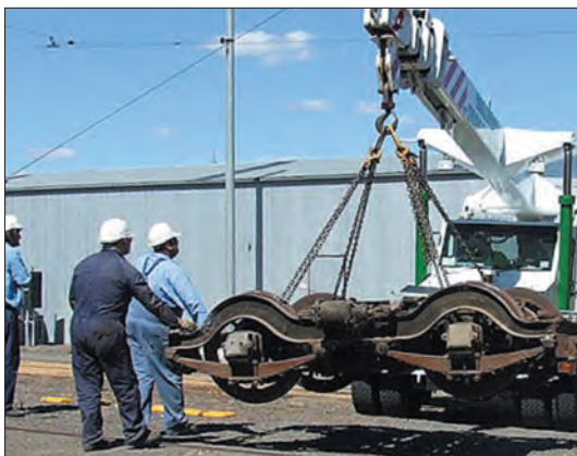
Anthony Smith, Alan Snowball, and Kym Smith assist with the movement of a No. 9 truck from the former bogie storage road to the main line.
