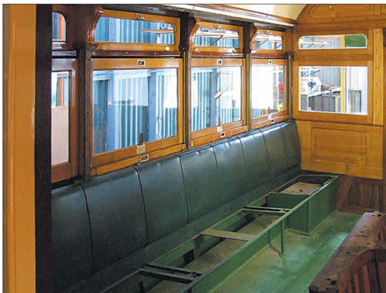
Windows, louvres, capping timbers, and seat backs reinstalled in the saloon of L 103.
