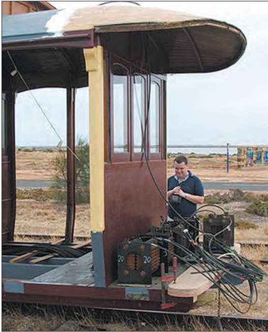
Stephen Parker examines the resistance banks temporarily located on the rear platform of tram No. 15 while it undergoes trials. Chris Summers
