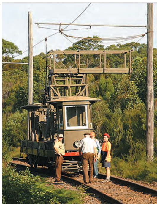
Ballast motor / overhead line car 99u on the Sydney Tramway Museum's Royal National Park line for some overhead wiring adjustment work on 14 April 2007.
