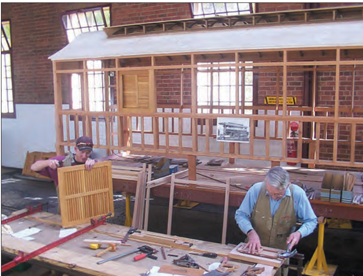
Luke Jenkins and Keith Trounson at work on the reconstruction of battery car No. 3. Bendigo Tramways
