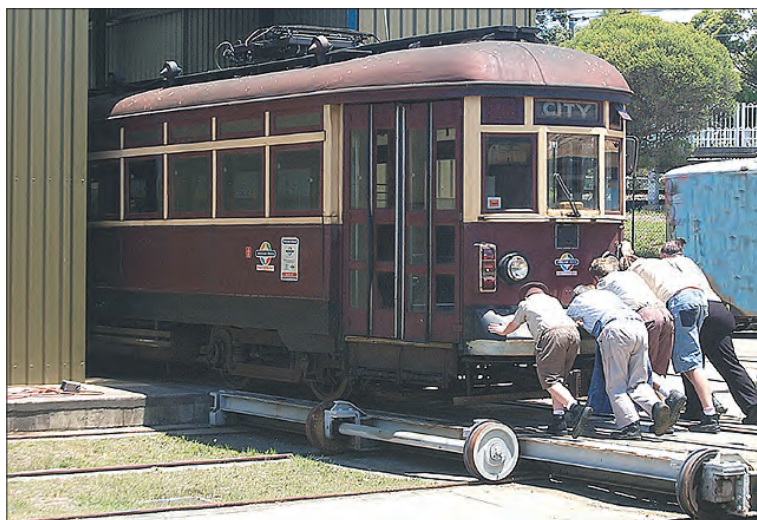
Car 358 being moved from the traverser into the workshop.
