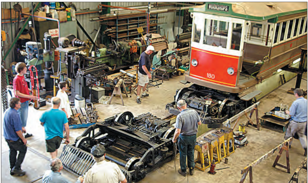
Reassembling the bogie for Brisbane 180. From left are Bill Denham, Vic Solomons, Bill Parkinson and Mick Duncan.
