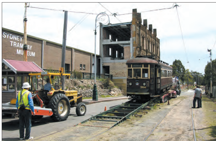
H Car 358 is assisted down the ramp with our tractor attached to the front and Mario's truck winch attached to the rear.
