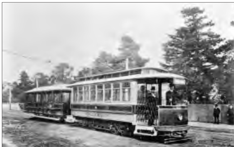
NMETL's single truck saloon car 9, one of ten cars built by J.G. Brill and assembled by Duncan & Fraser in 1906, is seen towing a crossbench trailer (one of 10 built by Duncan & Fraser in 1906 and numbered 51-60) in Fletcher Street, Essendon in 1907. The ten saloon cars became U class 202-211 under MMTB ownership.
