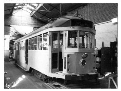
SW2 275 in undercoat in the paintshop, undergoing a minor overhaul and transformation into Bendigo Tramways No. 33.
