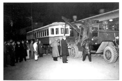
Car 1988 has been loaded onto Pittman's special trailer at Commonwealth Engineering, Granville for delivery to Randwick via Haberfield.
