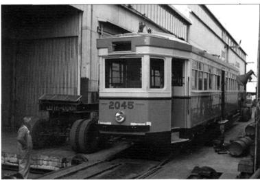
The car has moved from the traverser, foreground, onto Pittman's trailer. The back of the trailer will be jacked up and the bogie road wheels at left will be moved into position to support the rear end of the trailer.
