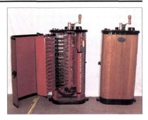
The two K35JJ controllers recently overhauled for use in Melbourne. Bendigo Tramways
