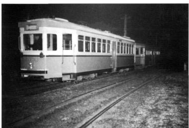
An unidentified R class car towed car 1988 from Haberfield to Randwick. Two kerosene tail lamps were attached to protect the unlit car during the journey. It is seen here being propelled along the right-of-way adjacent to Alison Road towards the workshop gates. The R car will leave 1988 in the workshop yard before returning to its home depot.
