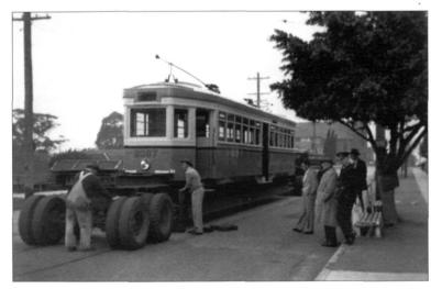
2087 is being delivered from Granville by Pittman's special trailer to Lane Cove terminus on 17 September 1953. Pittman's crew are removing the rear road bogie so the rear of the trailer can be lowered and the tram run onto the terminus track. John Burgess
