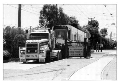
Melbourne three-unit Combino car 3520 is being prepared for unloading from the trailer which brought it from dockside to Preston Service Centre. Deliveries of the five-unit cars have now commenced.
