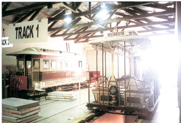
The three-track depot can house three grip car and trailer sets and in addition to the operating cable set also houses cable trailer 171. Ian Saxon
