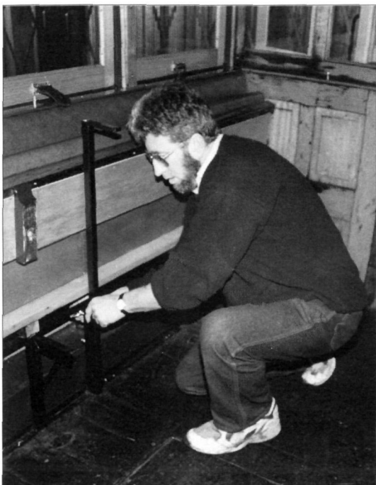
Steve Lea fixes the brackets against the upturned seats in the end saloon.
