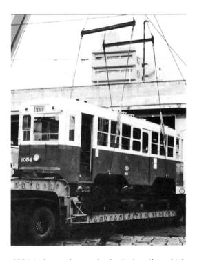
1054 is lowered onto the lowbed trailer which will take the tram to Hadaka. On arrival at the port, it will be prepared for the sea voyage to Sydney. Car 704 ex-Tokyo can be seen on the right.
