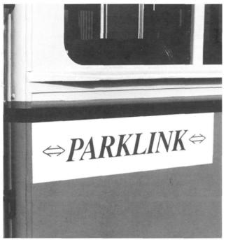
Cars used on the Parklink service (R class 1740 and R1 class 1979) carry magnetic rubber signs to indicate this special use. The signs are easily applied and removed, and do not spoil the paintwork.
