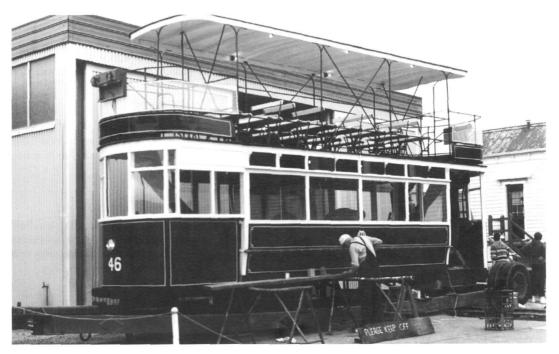
The lights are working and the last signwriting is being applied. Hobart double-decker 46 nears completion at Glenorchy. The final work was carried out with the tram sitting on the trailer which would take it into the Elizabeth Street Mall for the tramway centenary celebrations.
