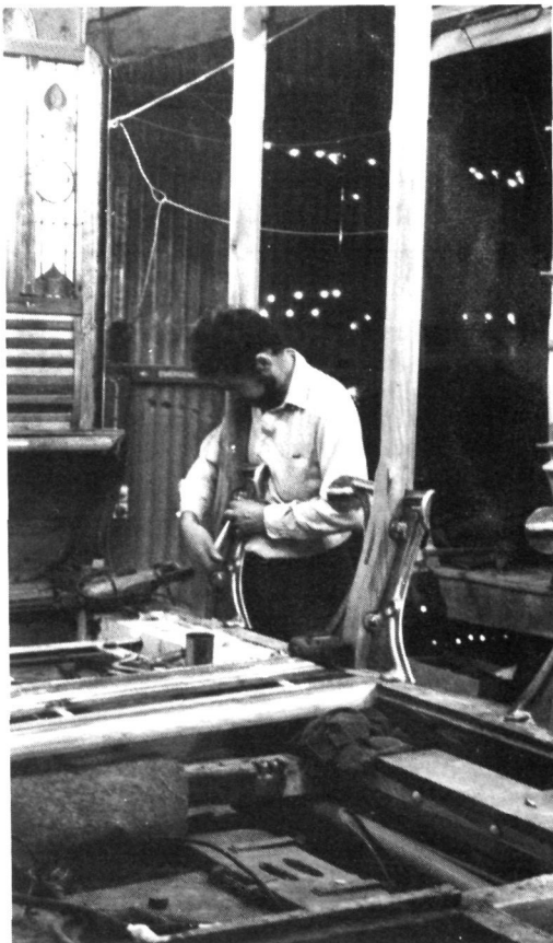
Right: Jack Pennack bolts a cast aluminium seat end to one of the new pillars on Car 42.
