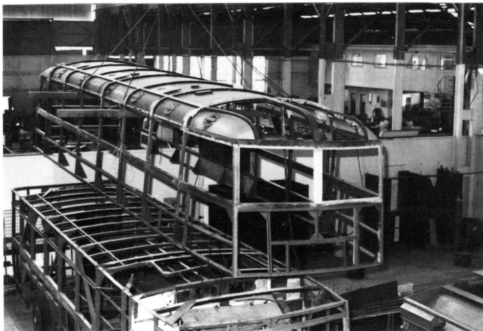
The top deck is united with the rest of trolleybus 19 at the STA/UTA Apprentice Training College. This year should see the body panels being applied and flooring replaced.
