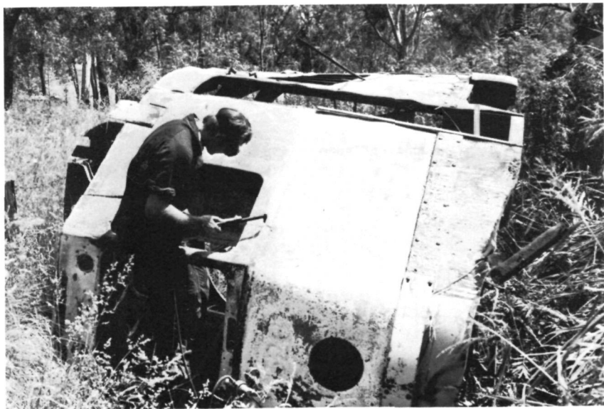
Mike Giddey at work cutting away the front apron of the remains of Four Motor car 526 at the Boonah tip.
