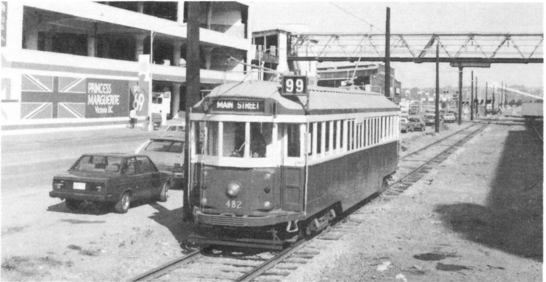
Ex Melbourne W2 481 passing Pier 69 on its journey to Main Street. The Ohio Brass single chime air whistle is located to the left of the destination box. The two road carbarn can be seen in the distance.
