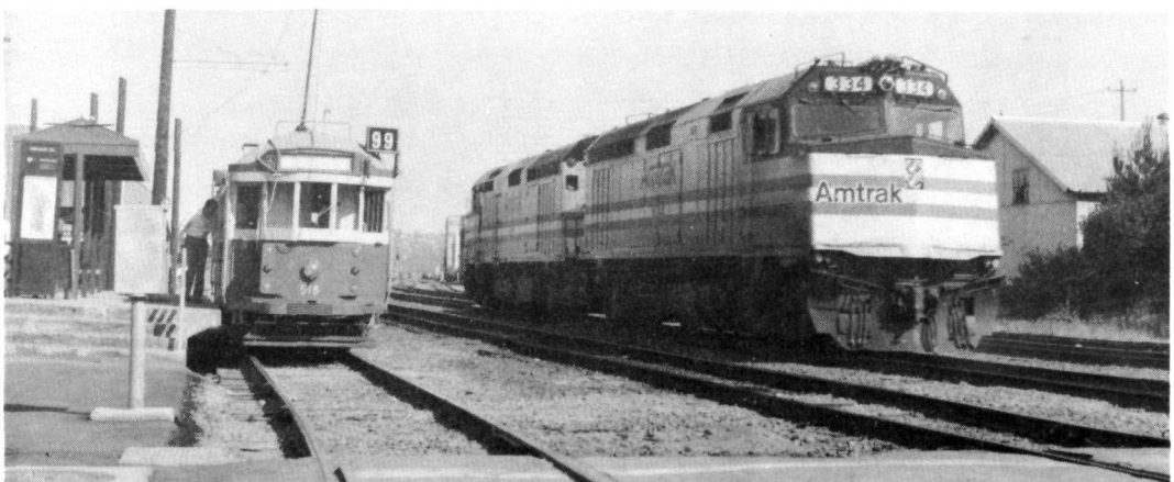
W2 518 at the Broad Street terminal being passed by two Amtrak EMD F40PH diesel electric locomotives on 11 June, 1982.
