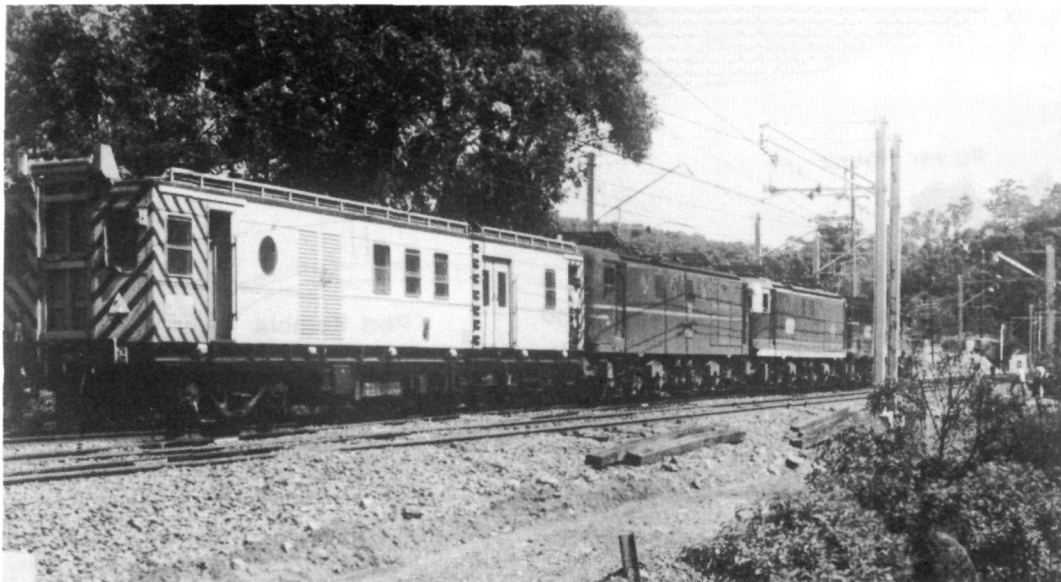
Overhead testing on a newly wired line. Locomotive 4403 towed electric locomotives 4608 and 4631 and overhead inspection car AL21 for unpowered testing of overhead wiring between Waterfall and Helensburgh on 15 March, 1984. The electric service to Helensburgh is expected to open in early May as the first stage of the Illawarra Electrification project.
