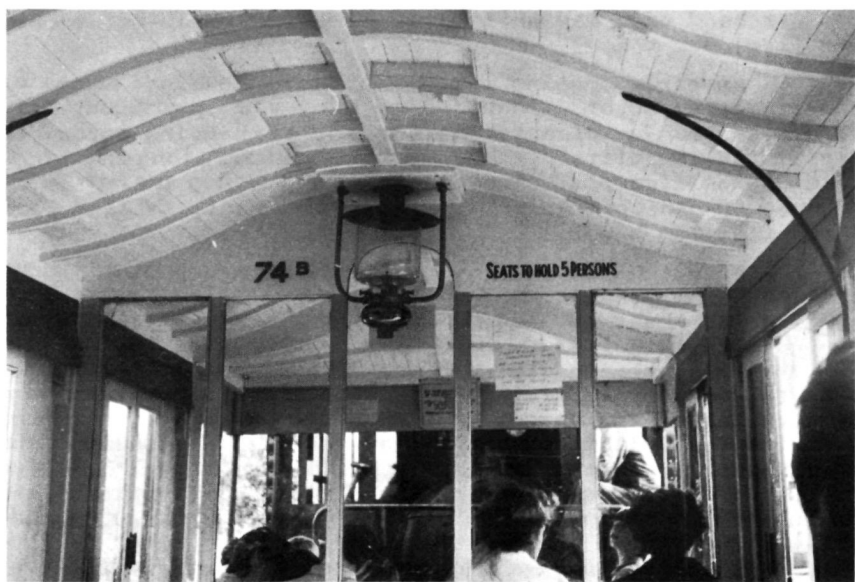
Interior of steam trailer 74B showing the kerosene light fitting. The roof brackets for the Hold-on straps for standing passengers can just be seen.
